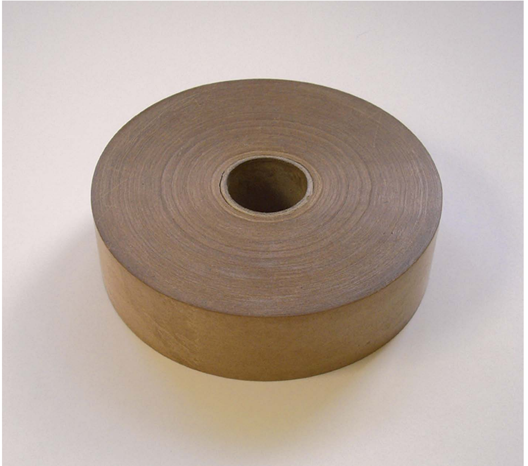
A roll of paper tape gummed solid after being stored in a damp workshop, (shown to size).
